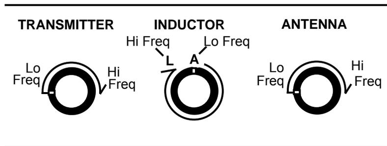
[ ] When tuning a T-network, start with a little more capacitance (tighter coupling) than you might actually need for your final match. Tighter coupling reduces the chance of arcing. Some users have suggested pre-setting capacitors fully meshed (0) for 160 and 75 meters, 3/4 meshed (2.5) for 60-20 meters, and 1/2 meshed (5.0) for 20-10 meters before starting to tune.
