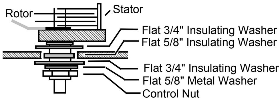
**Diagram 11: Capacitor Mounting**
