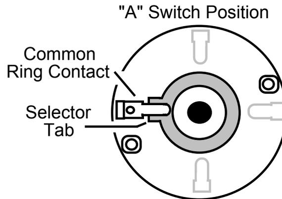
**Diagram 13: Switch Alignment**
