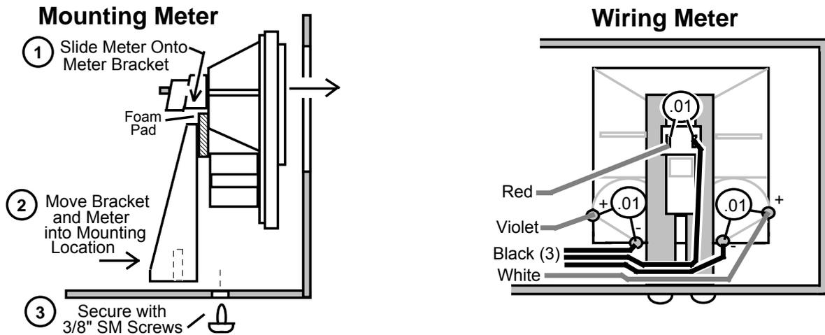
**Diagram 9: Meter Mounting and Wiring**
