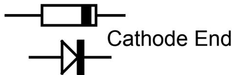
**Diagram 1: Diode Orientation**
